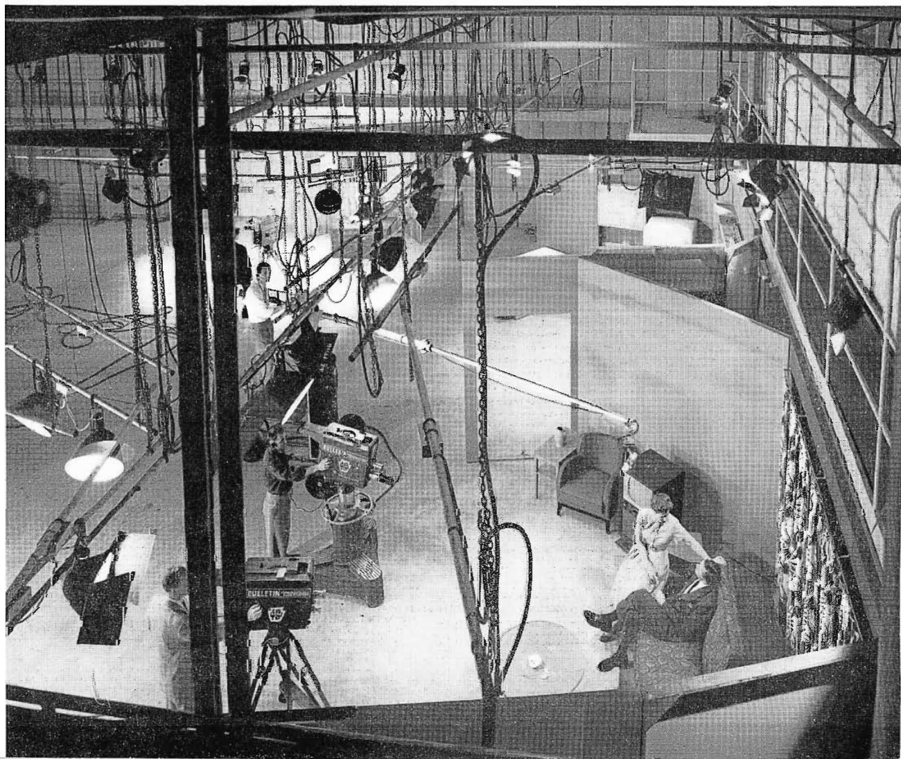
FIG. 21 (above). The large floor area of Studio No. 2 accommodates six 24-foot sets. In most cases all of the sets required for even an elaborate show can be set up beforehand, so that cameras simply move from one to another as action progresses. Because the cameras are in the center area they never have to be moved very far.
