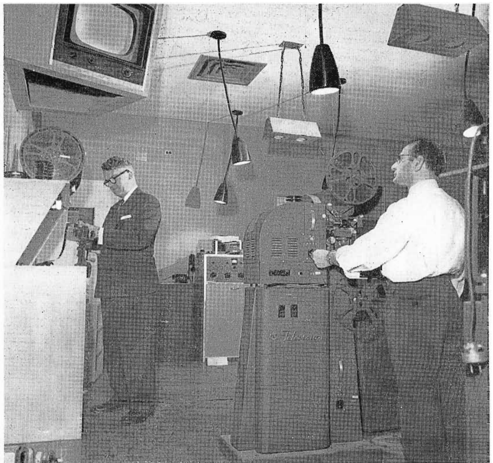
FIG. 47. View of part of the projection room in the WCAU building. There are three film cameras and two "live" cameras in this room. Floor layout is shown in Fig. 46 (opposite page). Three 17-inch receivers, mounted overhead at left, are used as monitors on film camera pickup. Monitor speakers associated with each projector-camera group are suspended from the ceiling so that projectionist can hear the sound pickup above other room noises.
