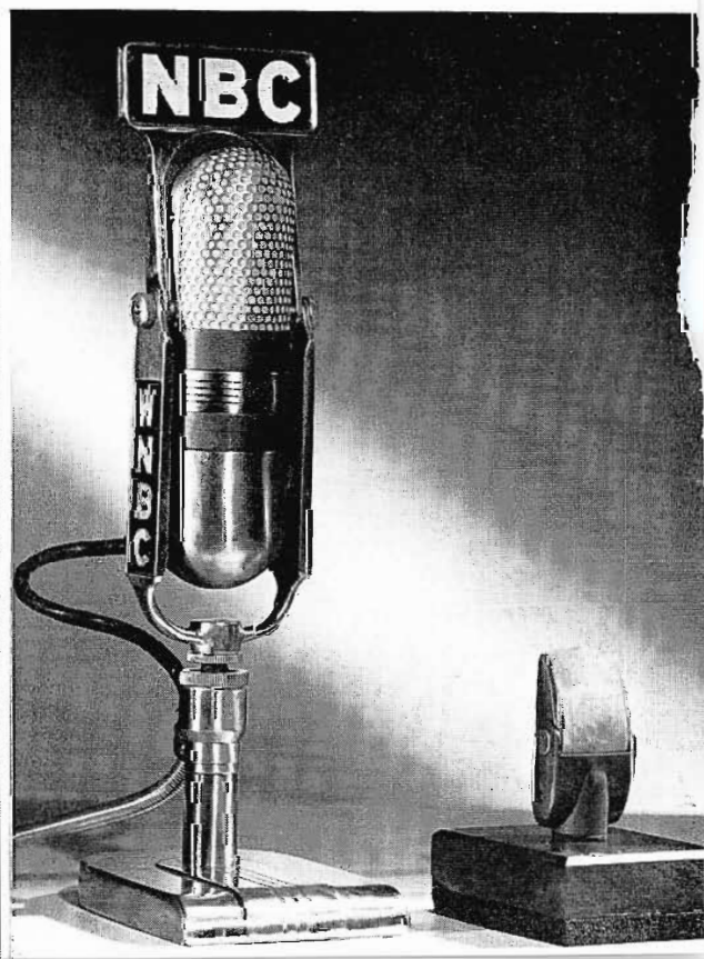
FIG. 7. RCA 77-D microphone compared to the RCA KB-2C for desk mounting.
