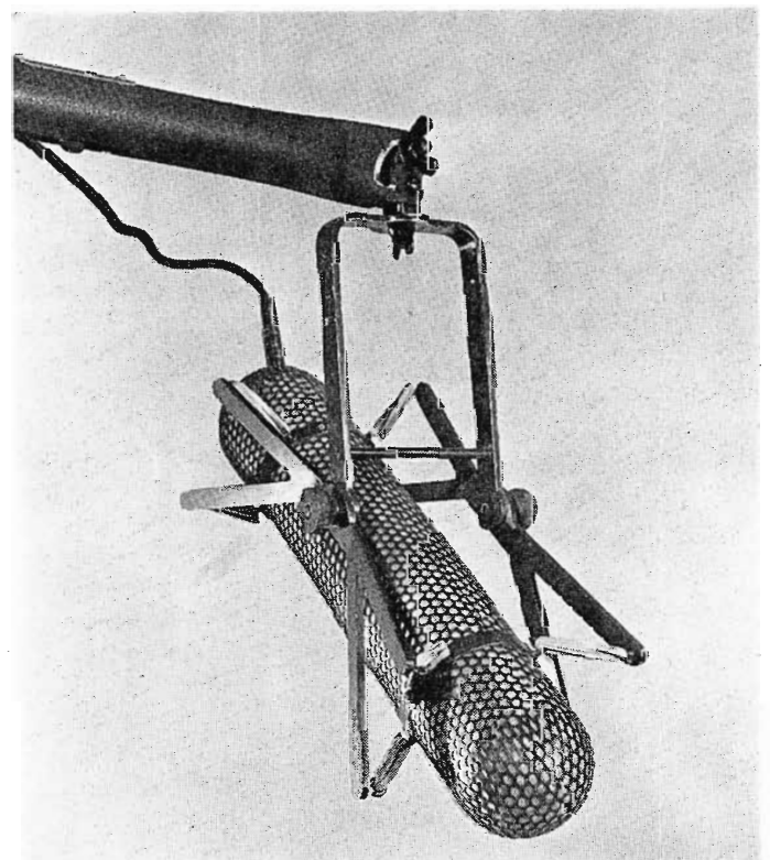
FIG. 4. Experimental highly directional gradient microphone—boom mounted—developed by Olson, Preston and Bleasey of RCA.
